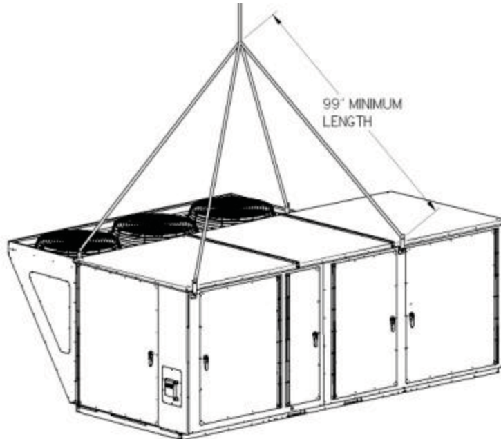
Figure 9 - Lifting Details of a 6-25 and 30 ton Energy Recovery Wheel or Power Return Unit
