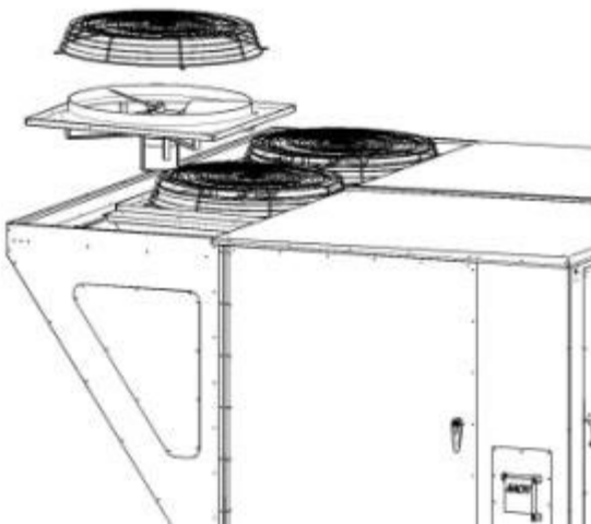
Figure 44 - Removal of a Condenser Fan Assembly
